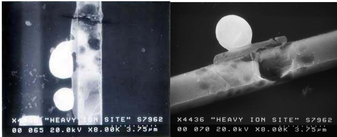
Figure 3.1. (a) SEM photograph of metallization failure induced by latchup after the silicon nitride layer was removed. (b) SEM photo of a region damaged from current during latchup where the metallization line remains conductive even though metal has been ejected from over 90% of the conducting metal line. [49].
