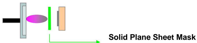
Figure 3.2: Target-shadow mask-substrate arrangement used to block out the ballistic particulates formed during target ablation.
