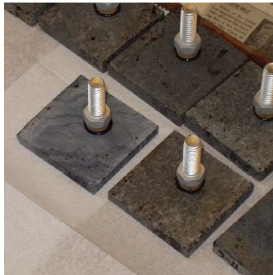
Figure 27. Photograph of Pull-off Test Method Specimens: Limestone and Diabase Substrates
