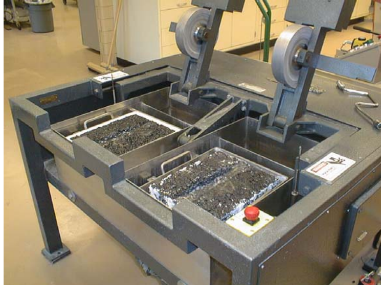
Figure 7. Hamburg Wheel-Tracking Device
