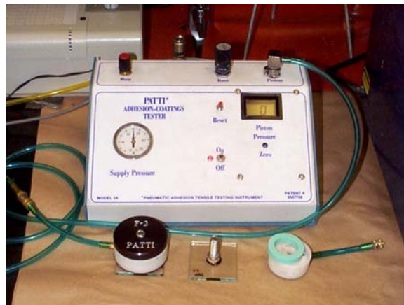
Figure 9. Photograph of Pneumatic Adhesion Tensile Testing Instrument (PATTI) and Associated Equipment
