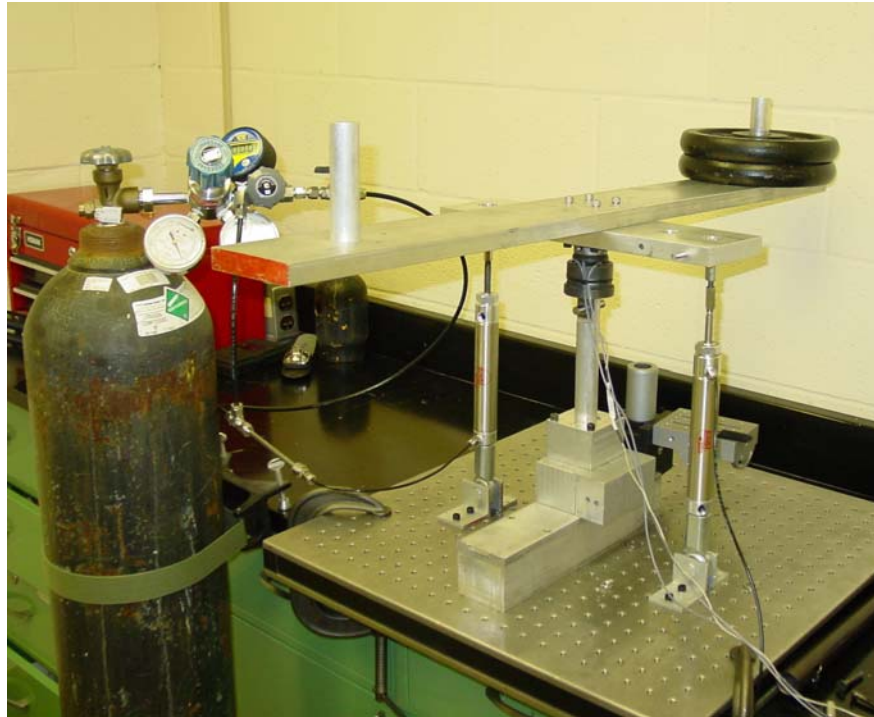
Figure 4-1. Three axis socket load cell calibration setup
