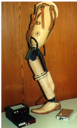
Figure 1-5. Electromagnetically actuated powered knee developed by Popovic with a battery pack.
