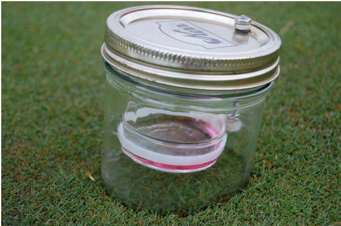
Fig. 1. Apparatus used for in-field ammonia volatilization estimates.
