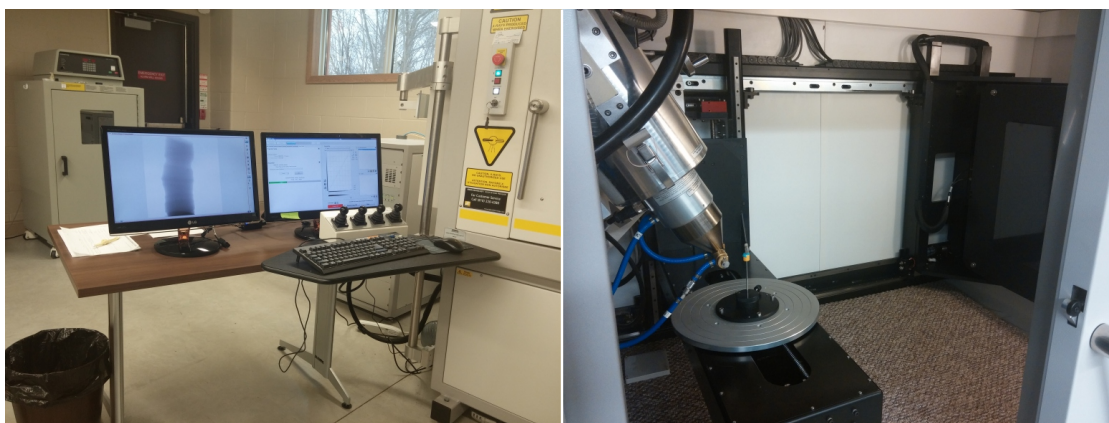
Figure 4.4: Nikon XTH 225 ST Micro-CT scanner, operated by Dr. Andrew Nelson (Sustainable Archaeology, The University of Western Ontario).
