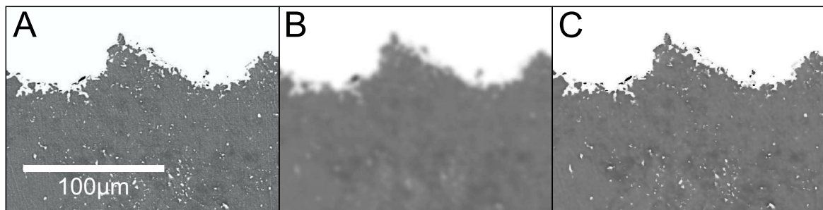
Figure 4.18: Gaussian filtering blends the entire image evenly, whereas bilateral filtering blends regions based on spatial and intensity sameness, resulting in decreased noise with preserved edge features. (A) unfiltered sample region of Eridophyllum ; (B) Gaussian ( \sigma_d=5 ) filtering applied; (C) Bilateral filtering ( \sigma_d=5 , \sigma_r=75 ) applied.
