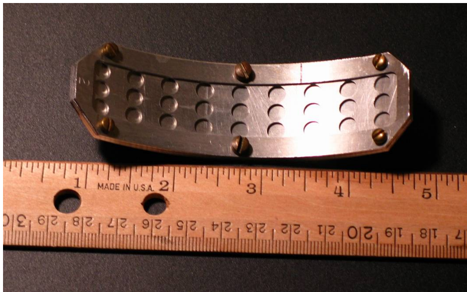
Figure 5.2. Example of sample holder specifically designed for the UNAM projects
