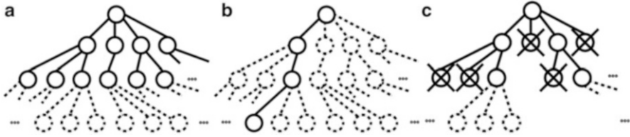
Fig. 1 Different tree search strategies in comparison. Dotted nodes are yet to be explored. Crossed out nodes are pruned and will not be branched. (a) Breadth-first-search (BFS). (b) Depth-first-search (DFS). (c) Beam-search (BS)
