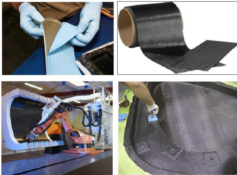
Figure B.6: Prepreg sheet, roll and lay-up [140-143]
