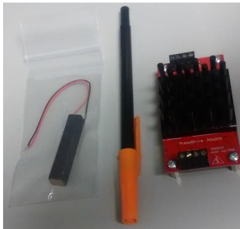
Figure 5.6: PiezoDrive Piezo stack actuator with the voltage driver board
