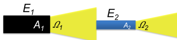
Figure 3-16: The etendue is determined by the emission area of a source and the solid angle of the light cone. For example, 100% of the light would pass from one section of the system to the next one if the ratio of their etendues ( E_2/E_1 ) was 1.
