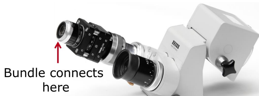
Figure 3-11: The bundle adapter is connected to one of the microscope oculars and it captures an image at the ocular's image plane.
