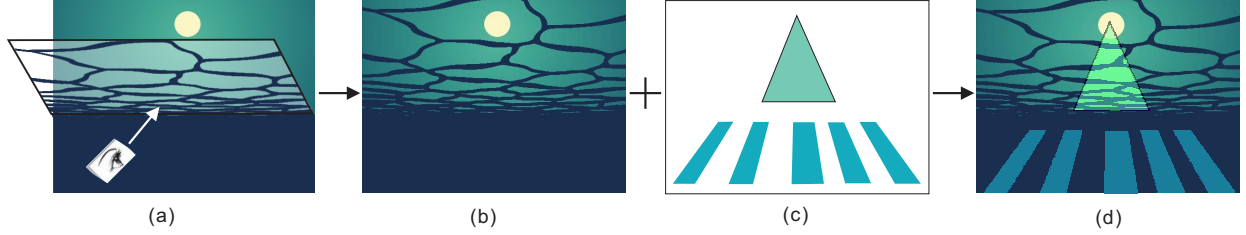
Figure 2. Water caustics model. (a) A scene composed of the water surface and the background image surface. (b) Projection of the scene on the view plane. (c) Image of light scattering effect. (d) Blending of the projected image and light scattering effect.
