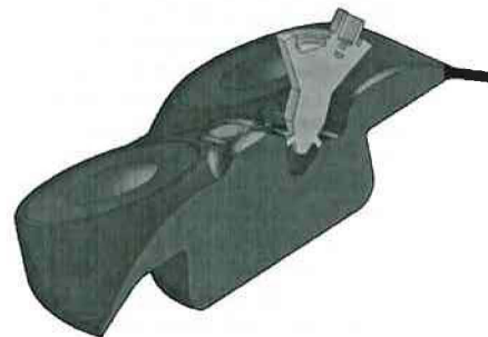
Fig. 3 Plane cut of the in-cylinder and PC volumes
