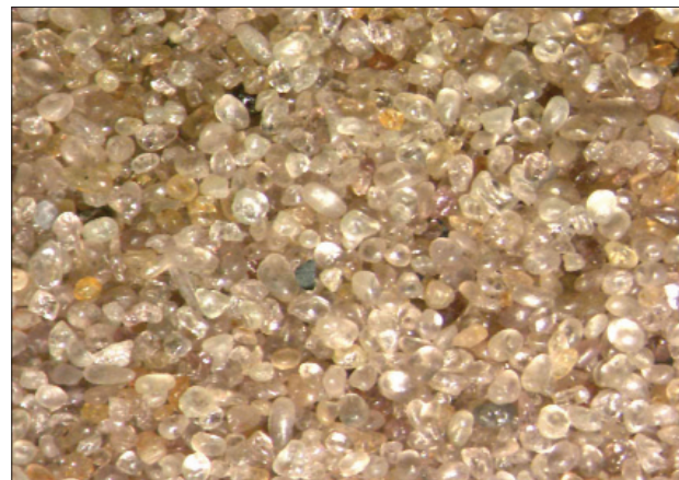
Figure 6—The sink fraction of -250+150 \mu\text{m} zircon at 4.45 initial separation relative density
