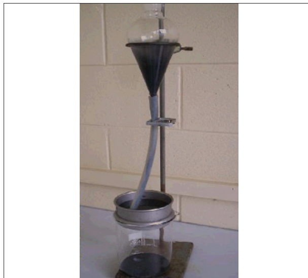
Figure 2—Removing 'sinks' fraction through a clean sieve
