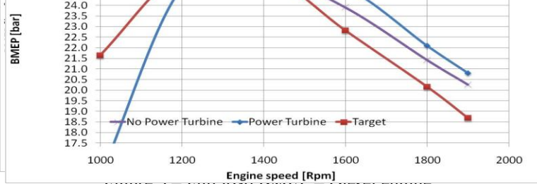
Figure 5 – Full load BMEP – Diesel engine.
