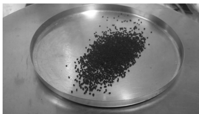
Figure 7. SAP after dewatering brown coal. Note increase in size and the dark colouration afforded by traces of humic material adsorbed onto the alkaline SAP.
