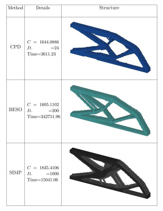
Table 4.3: Topology optimization for a cantilever beam  $(120 \times 50 \times 8)$
