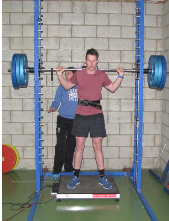
Figure 4.2. Participant preparing to perform the half-squat protocol on the BMS with the LPT attached to the squat bar.
