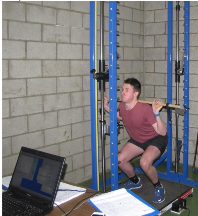
Figure 4.2. Participant preparing to perform the half-squat protocol on the BMS with the LPT attached to the squat bar.
