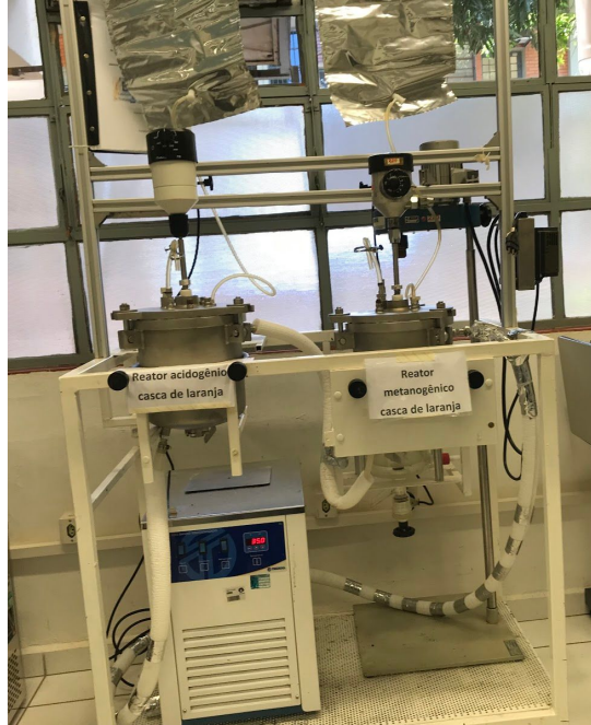
Figure 1: Two Stage Reactor Configuration
