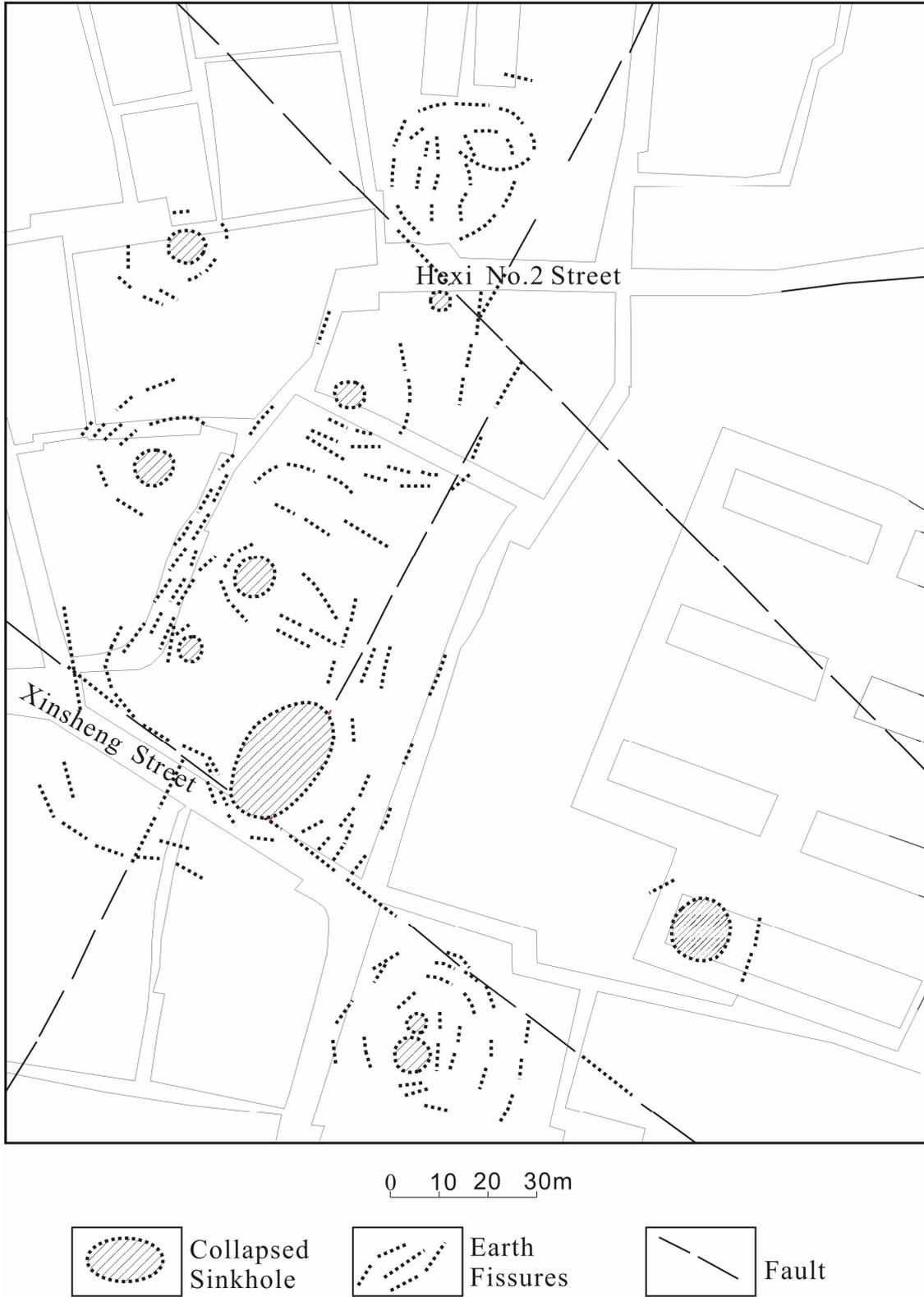
Fig.2 Karst sinkholes and earth fissures in Xuzhou City
