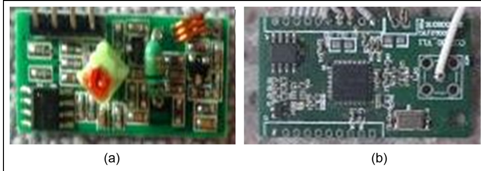
Figure 7. (a) A 315-MHz module and (b) a ZigBee module.
