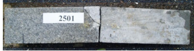
(b) interface cracking and kinking into rock (IR)
