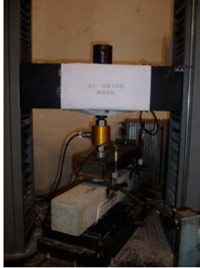
Figure 3: Experiment setup for four point shear test.
