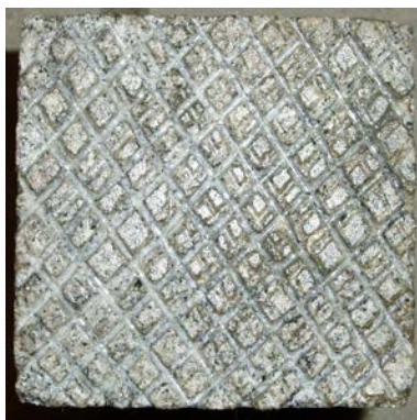
Figure 2: Roughening of rock portion at the interface.
