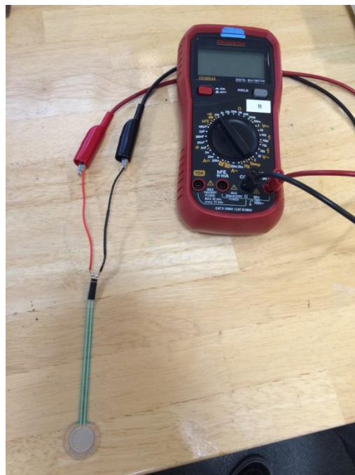
Figure 27: Setup for pressure testing.
