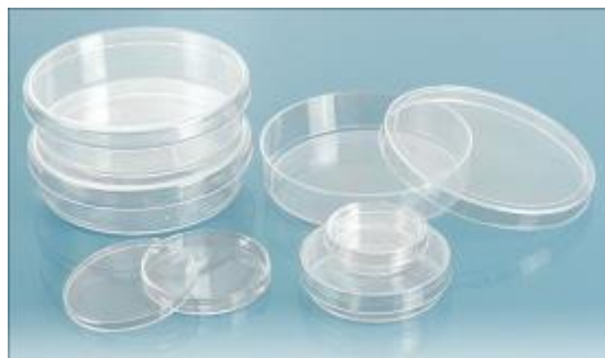
Figure 5. Variety of petri dish sizes that can be used for hanging drops.
