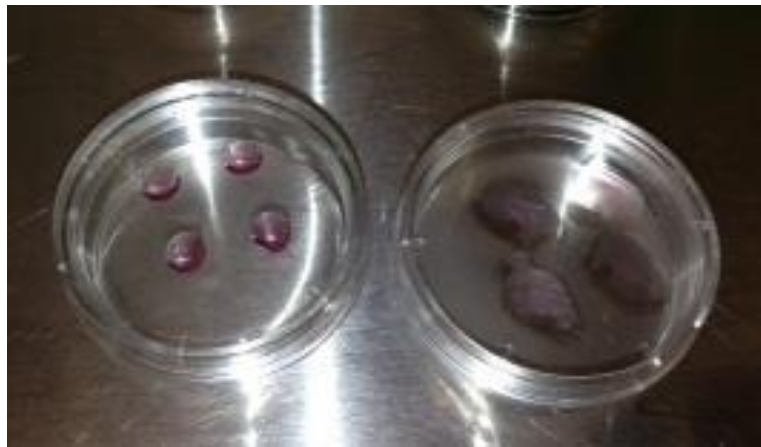
Figure 26. PDMS-coated petri dish on the left vs. non-coated petri dish on the right
