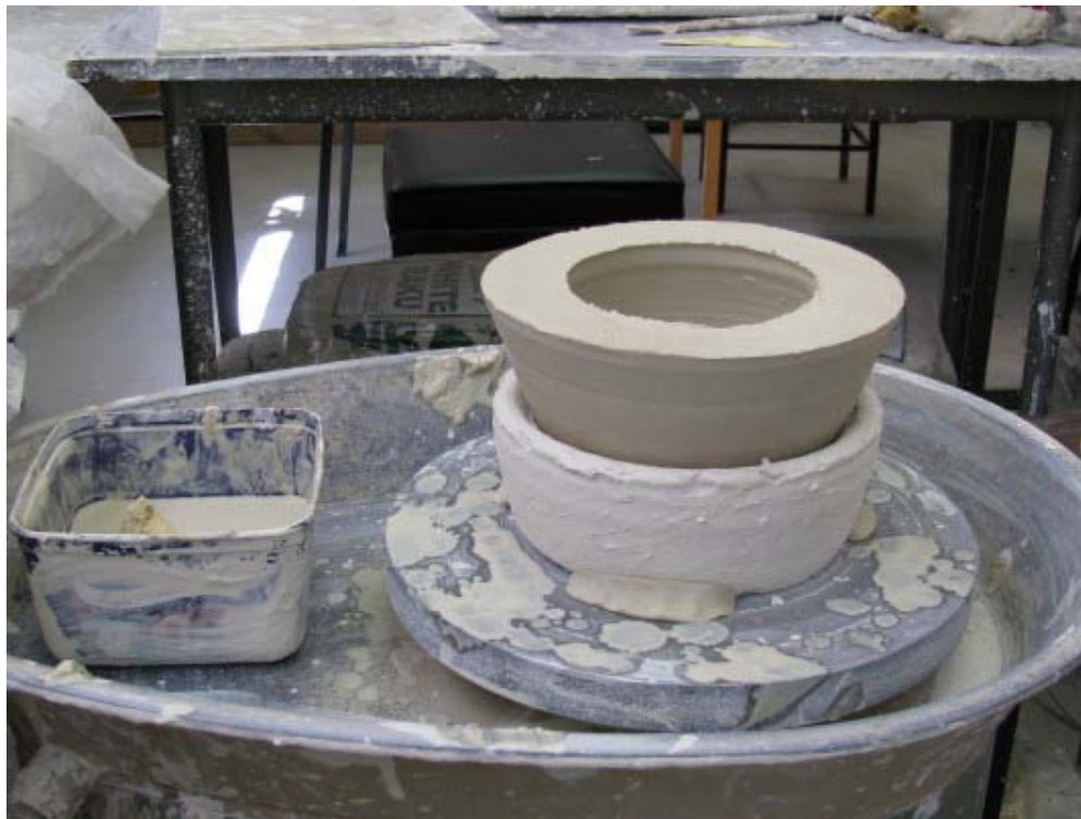
Form is inverted in chuck to complete throwing.
