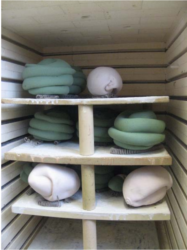
Glazed pieces are loaded into kiln with other volcanic glaze forms. As they are glazed all over, they are fired on old electric kiln elements.
