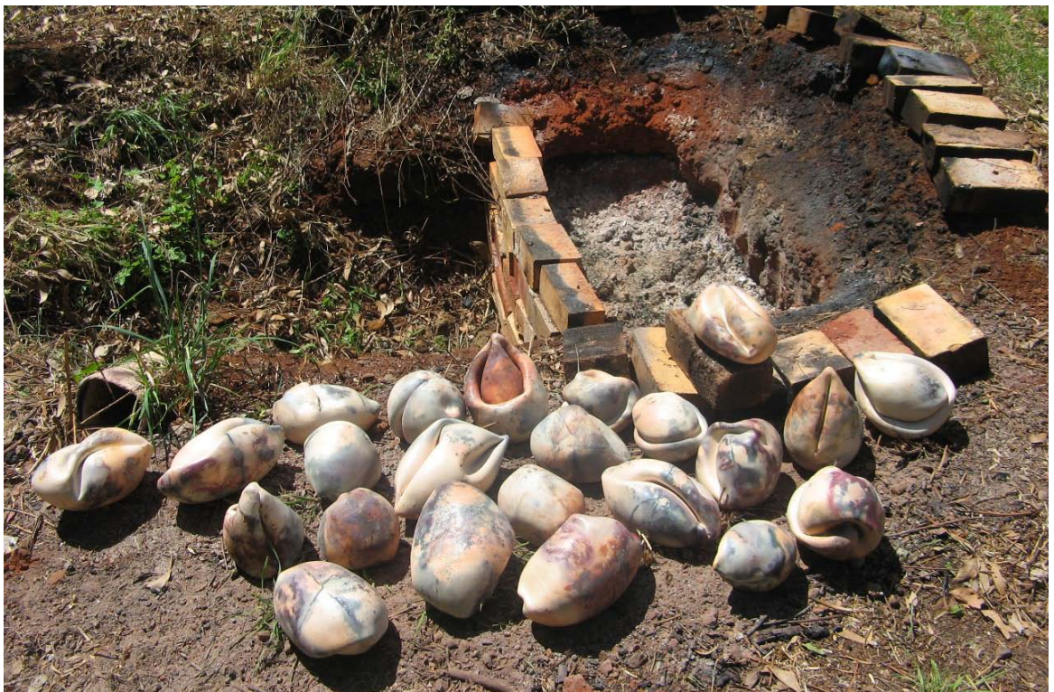
Forms are removed from pit and cleaned with soft damp cloth.
