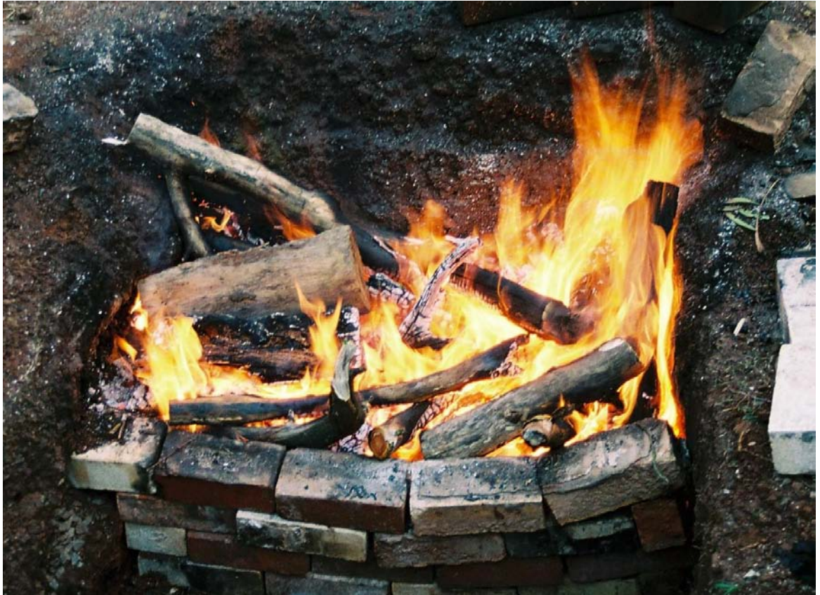
Pit is filled with wood, set alight, and continually stoked until an even distribution of embers is present.
