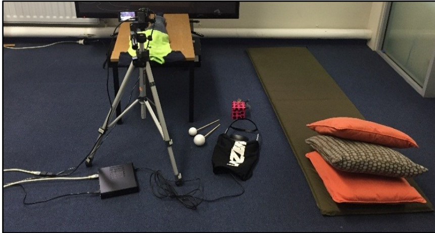
Figure 1. Experimental set-up. The participant lays down on the mattress beside the video camera and table while wearing the HMD goggles. The participant would then see the world from the doll's perspective.
