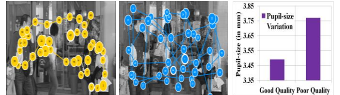
(a) eye-traversal for good quality video contents (b) eye-traversal for poor quality video contents (c) pupil-size vary for good and poor quality
