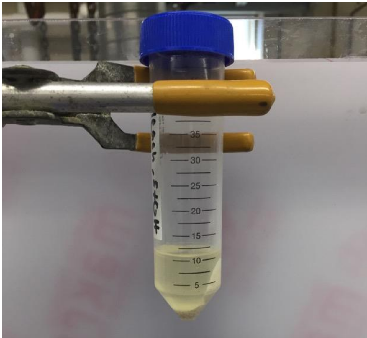
Figure 34: Eggshells, Bleach, 24 hours, 1.0 g catalyst, EtOH, Stirred, 27 hours.
