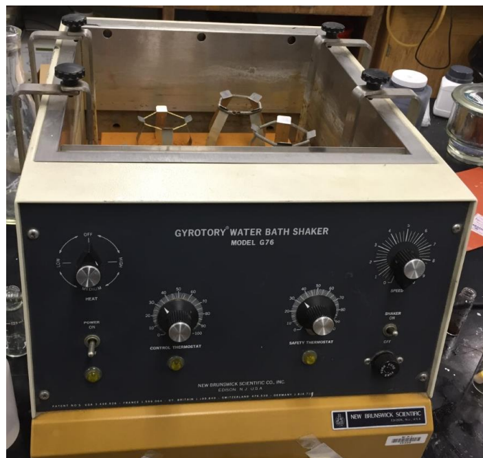
Figure 10: Oscillating Water Bath
