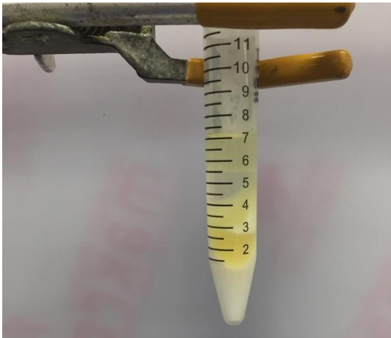
Figure 27: Eggshells, 400°C, 6 hours, 900°C, 6 hours, 1.5 g catalyst, MeOH, Stirred, 22 hours.
