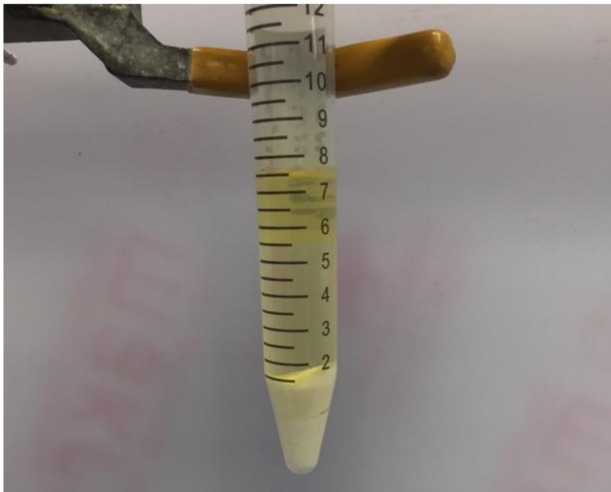
Figure 28: Eggshells, 900°, 1.0 g catalyst, MeOH, Oscillating Water bath (35°C), 19 hour.
