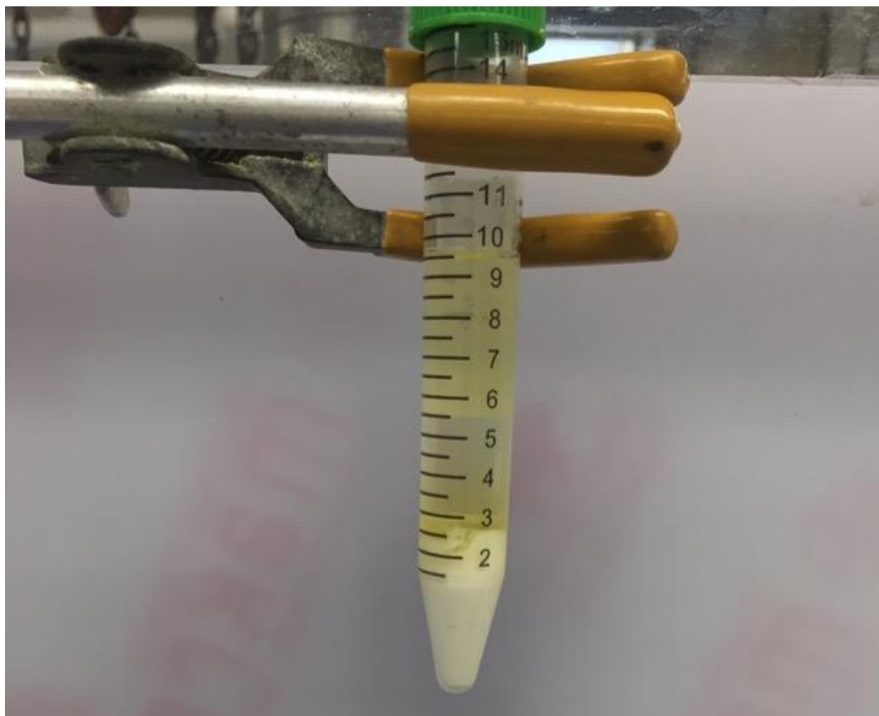
Figure 26: Eggshells, 900°C, 6 hours, 1.0 g catalyst, MeOH, Stirred, 24 hours.
