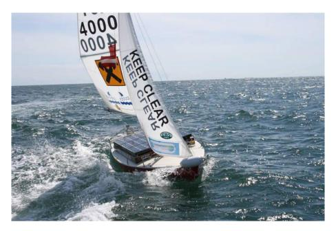
Figure 4: Roboat under sail ("Roboat: Home," 2013)
