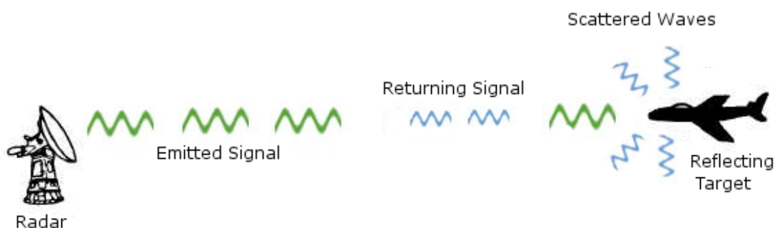
Figure 5: A basic depiction of a radar system detecting an aircraft. The emitted signal (large green waves) hits the aircraft and scatters in every direction (smaller blue waves). Some of the scattered signal returns to the emitter.
