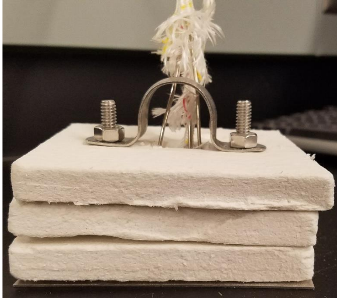
Figure 32: Constructed Final Plate Thermometer
