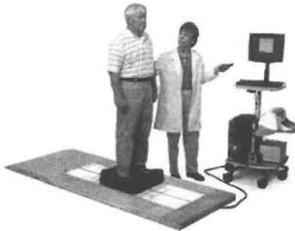
Figure 1. Subject standing on the posturography platform used for CTSIB (foam pad in place).
