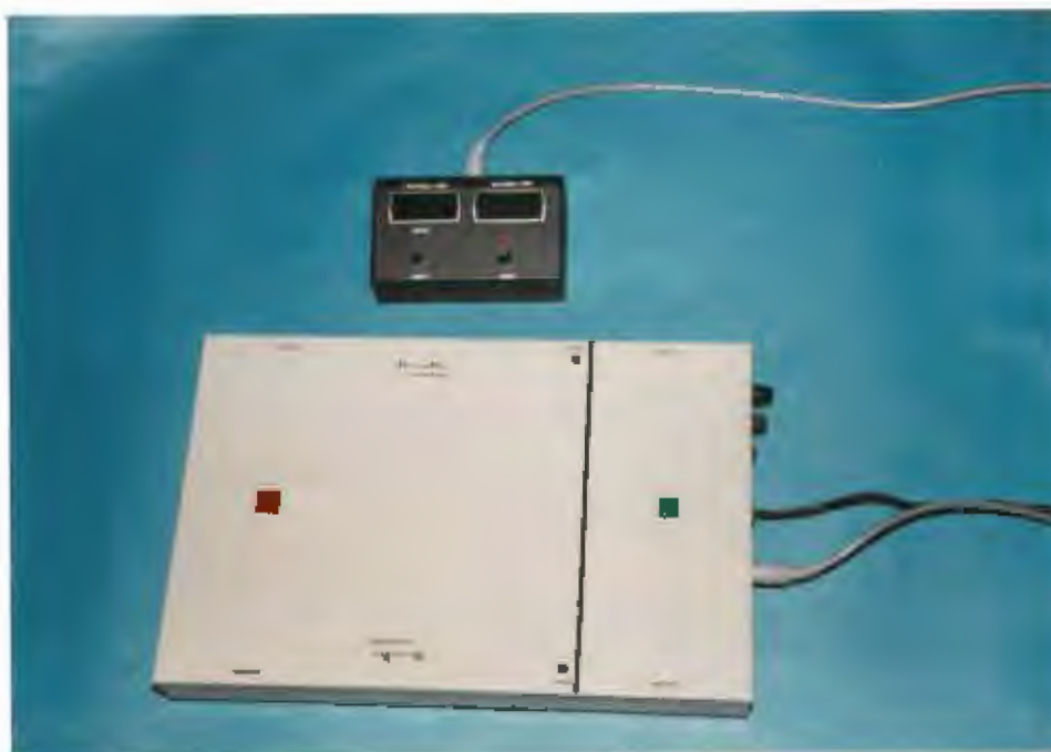
Fig.1b- The Reaction Plus was used in testing to measure the reaction, motor response, and total response times of the subjects.
