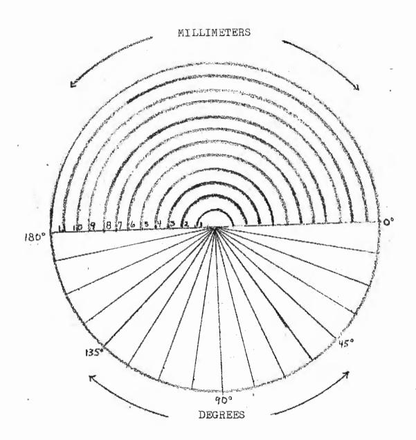
The reticule seen through eyepiece of the slit lamp as is used to measure degrees rotation of the truncated soft lens.
