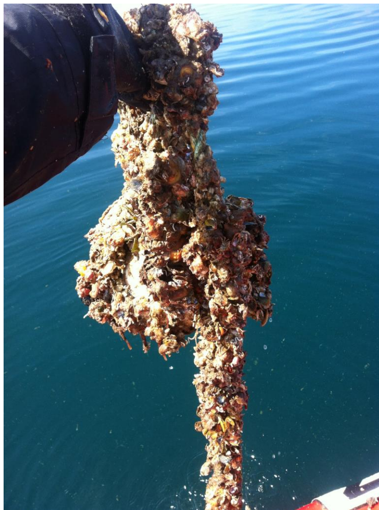
Figure S5.3: Biofouling of a mooring line and buoy 189 days after deployment. The tracking receiver itself was relatively fouling free, particularly the receiver head containing the hydrophone which had been painted with anti-foul.
