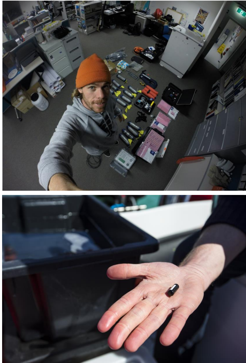
Plate 4.1: Top: Preparing acoustic tracking equipment before deployment. Bottom: A V9 acoustic tag used in detection range testing (Photo: Paul Jones).
