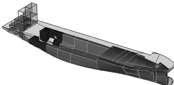
Figure 2: Simulated damage consisting of compartment groups NO°2, NO°1 and forepeak.
