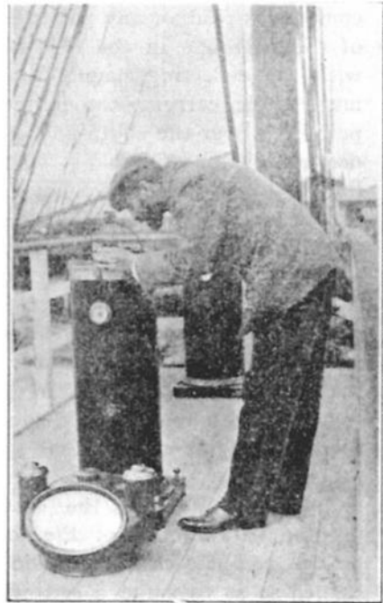
FIG. 4b. Showing how observations for horizontal intensity are made with the L. B. deflector.
