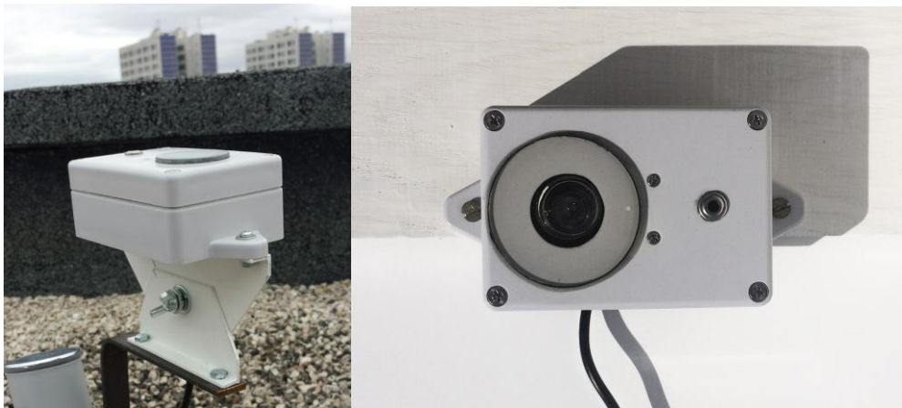
Figure 5. Possible installation of TESS photometer (left). It must be in horizontal position so the sensors point toward the zenith. You can also see the top view (right) and appreciate the brightness sensor on the left and cloudiness on the right.
