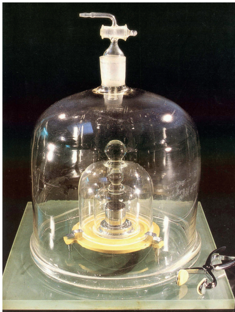
1: International prototype of the kilogram. Cylinder made of a platinum-iridium alloy, kept at the International Bureau for Weights and Measures (BIPM) in Sèvres, Paris. (Source: BIPM)
