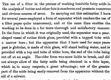
In using the apparatus, the soap obtained from any convenient weight of fat, but preferably from about five grammes, is poured into strong hydrochloric acid previously introduced into the separator, the residual soap being washed in through a funnel with boiling water.
