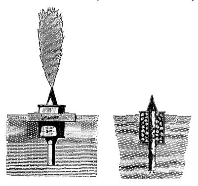
sugar; these chalk-lumps are then heated to a white heat in a crucible containing a certain proportion of phosphorus, which being converted into vapour by the high temperature, is absorbed by the chalk when at a white heat, much as a sponge absorbs water. The chemical material thus formed (phosphate of calcium) is, when cool, placed in the signallight-case, and the whole soldered down air-tight.
