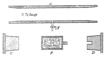
the tube before and after an experiment without touching it with the fingers. The plunger P is hollow and its ends perforated. It is loosely packed with glass wool dipped previously into  $P_2O_5$  powder. No  $P_2O_5$  is placed on the wool touching the ends of the plunger, and a glass sleeve similarly protects its sides.
