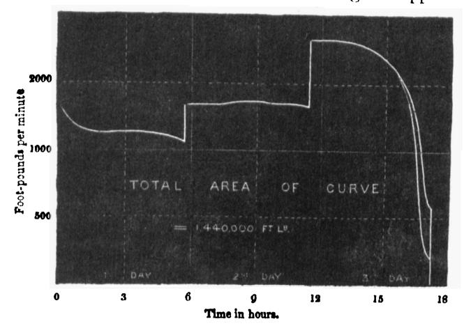
totally discharged, that there was still a large charge stored up; hence the numbers given above for the capacity are probably under the total value.
