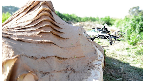
Figure 1 Off the shelf drones used for 3d scanning of structures at different stages of the construction.
