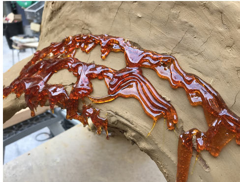
Figure 8 Robotic deposition of natural resin on the mud shell while the upper clay mix coating is still wet so both material adhere to each other. Different geometric areas of the mud shells are explored and chosen for the resin robotic pouring to test different finish.
