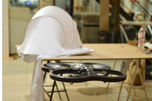
Figure 4 Parrot Drone performing the 3d scanning of the shell at its initial state by providing a series of photos around and on top of the structure.
