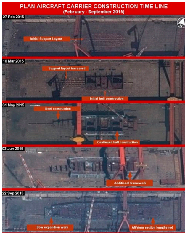
Graph 4. China's first domestic carrier under construction in Dalian shipyard
