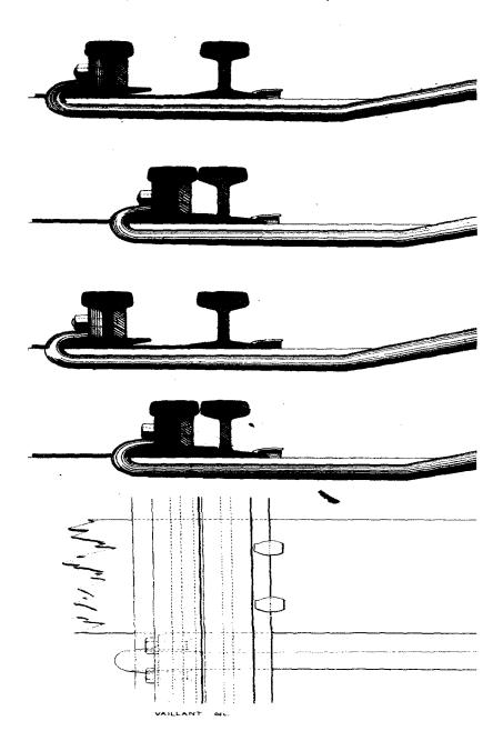
a positive motion, the first pair of wheels of a train on the main line moving in the proper direction of travel, closes the switch, that is, sets it for the main line.
