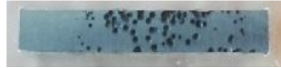
Figure 3: Tested in 1M KBr surface of specimen after polarization
