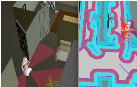
Figure 1: The robot enters a simulated apartment. On the left: the simulator. On the right: ROS standard navigation stack with sensory input from simulator.
