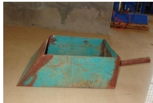
Fig.3 Device for pouring sand
