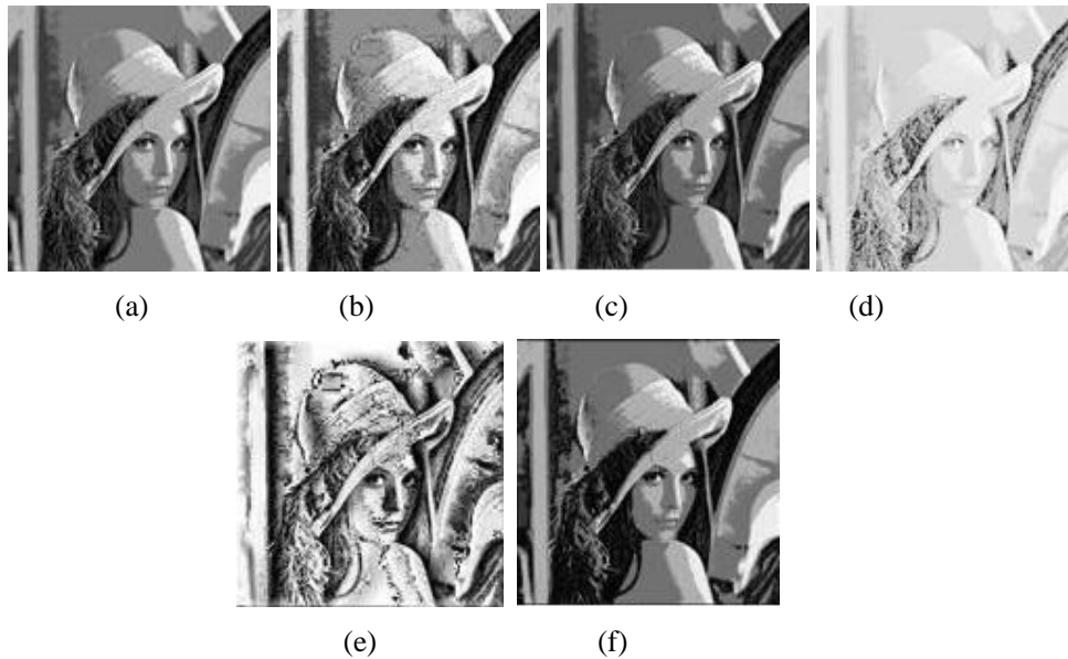
Fig 1: Results for Lena: (a) input Image (b) result of HE Method (c) result of power Law Transformation Method (d) result of Logarithmic Transformation (e) result of LHE Method (f) result after applying OBCS Method.
