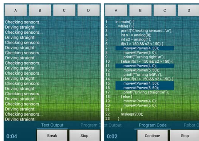
Figure 3: Two screenshots (cropped) from a debug session. Left: Standard output. Right: Setting breakpoints in the source code while the program is suspended.
